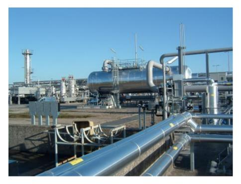
Pipeline specifications require removal of harmful acid gases carbon dioxide (CO2) and hydrogen sulfide (H2S) from the pipeline. H2S is highly toxic and corrosive to carbon steel. Carbon dioxide is also corrosive, reducing the BTU (British Thermal Unit) value of the gas. The natural gas desulfurization process can remove these acid gases, making natural a marketable product and suitable for transportation.
