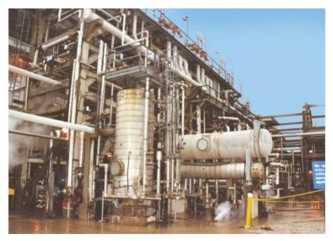
Heavy raw materials are generally difficult to process by FCC or reforming, but can be converted by hydrocracking. The feedstock is cracked by catalytic cracking in the presence of hydrogen, which produces a mixture of gasoline and distillate. There are about a dozen different hydrocracking processes in use.
