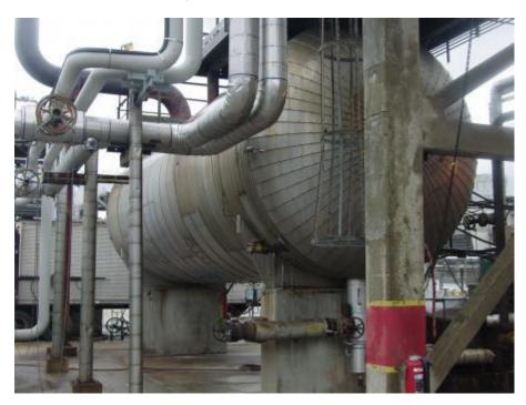
In the first stage of gravity separation, not all water is separated from crude oil. The water content of the separated crude oil may still be as high as 15%, and it is in the emulsifying state, so it is difficult to separate out again. The de-emulsification process is completed using chemical reagents and heating to eliminate the emulsifying state of oil and water in order to remove moisture before transporting crude oil.
